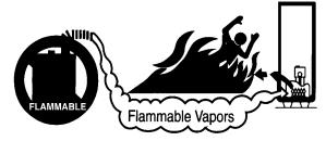
⚠Vapors from flammable liquids may explode and catch fire causing death or severe burns.
